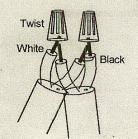
Connect the wires marked TO ORIGINAL THERMOSTAT WIRES on the new thermostat to the wires that were just disconnected from the screws on the original thermostat and stripped. Twist-connect the wires. Black connects to black, and white connects to white. The green wire may just be clipped out of the way. Check that the connections are secure and that there are no exposed wires.
