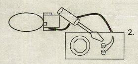
2. Next you will wire the new thermostat to the compressor. The wire leading to the original thermostat will be used for part of this connection. Unscrew this wire at the screw terminals in the original thermostat. Clip and strip ½ " on both the black and white wires.
