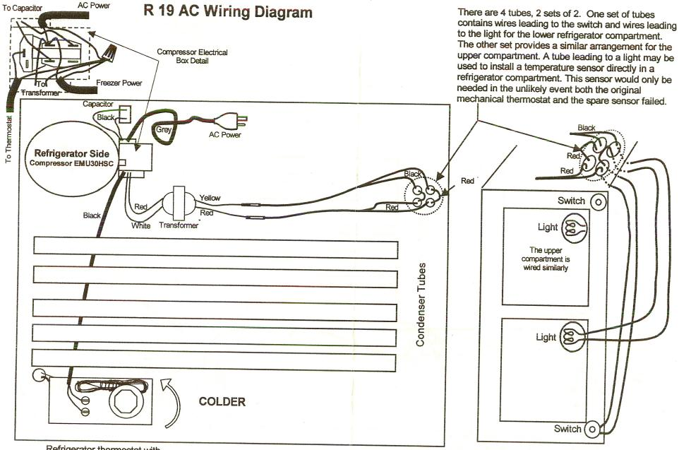
Refrigerator thermostat with spare temperature sensor (wound white wire inside) for use with an electronic replacement thermostat
